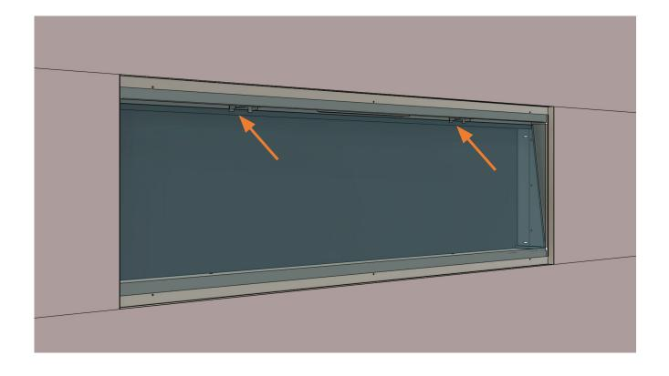
Place the decorative crystal or wood log media onto the fire bed, then reinstall the front glass – secure the glass by installing the bolt and hinge below the top trim
