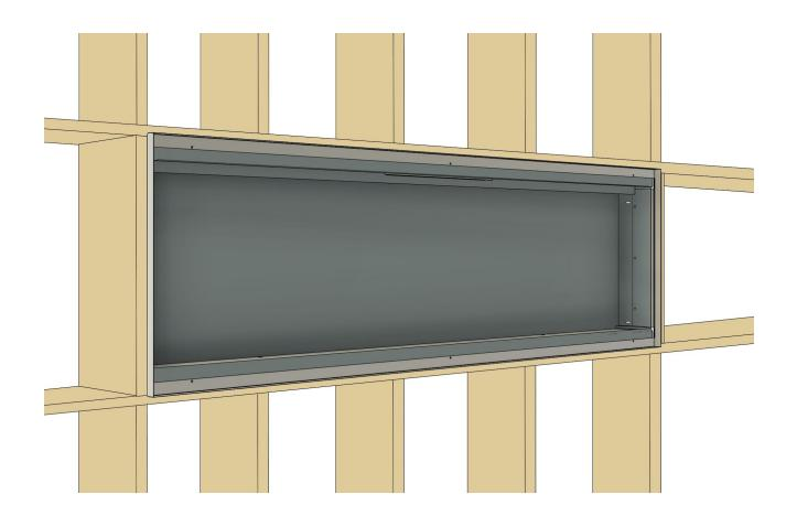
With the edgings strip installed, position the fireplace into the opening.
