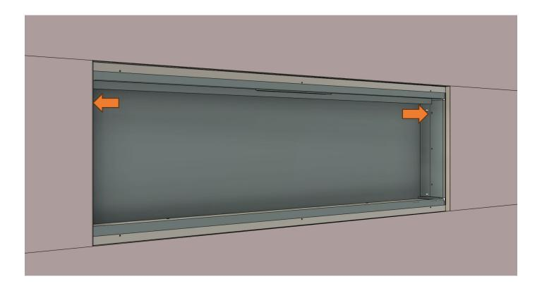
Secure the fireplace using the provided ST4x12 metal screws, insert the screws into the opening on the top left and right of the side panels. Ensure side panels do not deform when screws are inserted.
